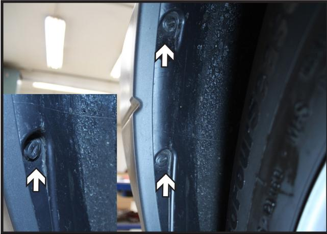
1. In the front wheel well using a straight screwdriver, turn the two (2) upper and one (1) lower fascia pins 90 degrees to unlock and remove. Both driver and passenger sides.
