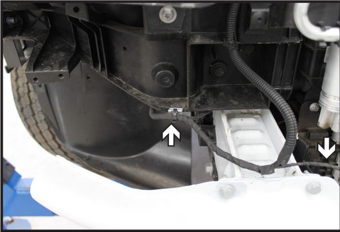
9. Remove the temperature sensor from bumper (right) then unhook clip from frame (left) and set aside.
