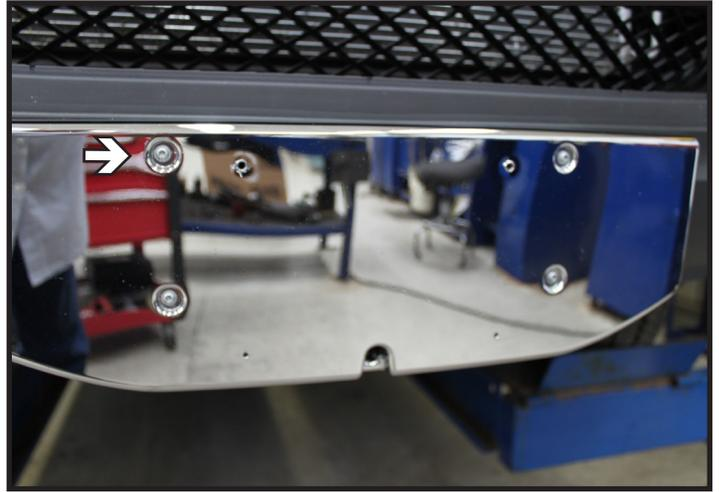
6. Using a 20 Torx remove the four (4) bolts and remove the license plate bracket.
