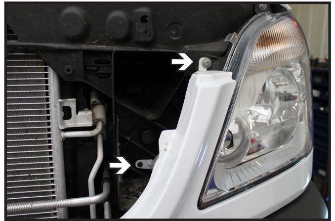
4. Remove the upper screw using a 27 Torx and lower screw using a 20 Torx on both driver and passenger sides.
