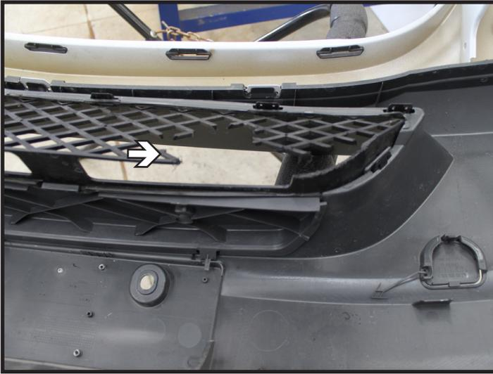
17. Hold front fascia up to frame and mark to cut out for clearance around baseplate. After cutting sufficient amount for clearance, re-attach fascia to vehicle.
