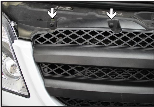
3. On top of the grill locate and remove the two (2) screws using a 25 Torx. Do this on both sides of vehicle. After the four (4) screws are removed the grill can be removed from the vehicle.
