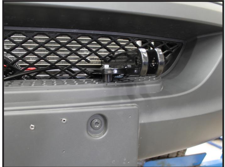
18. Use 3/4" spacertube before installing 8MM-1.25 x 50MM bolt and 8MM lockwasher, typical both sides.
